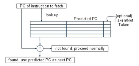
Branch folding buffer - an extension of the BTB, instead of keeping the predicted
